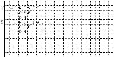
This is used to select the camera go back to "PRESET", "INITIAL", "PHASE" condition
